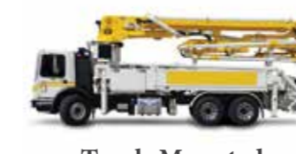
Truck-Mounted Concrete Pump
