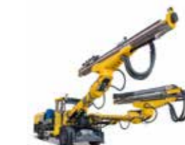
Face Drilling Rig (Jumbo)
